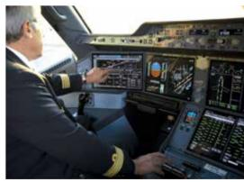
In December, China Eastern Airlines took delivery of the first A350 equipped with the new devices, which are designed to aid crew interaction, cockpit symmetry, and smoother information management. Some 20 airlines have selected the option for their new A350s. The touchscreens received EASA certification in November 2019.
